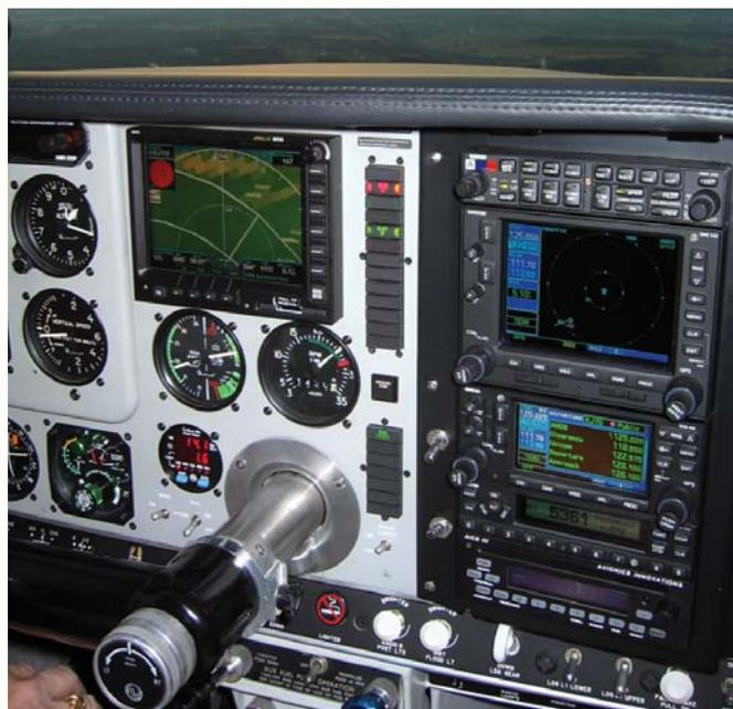
The panel of N1733G was built using the new Fast Stack Pro Hub and cable system designed by Approach Systems.
